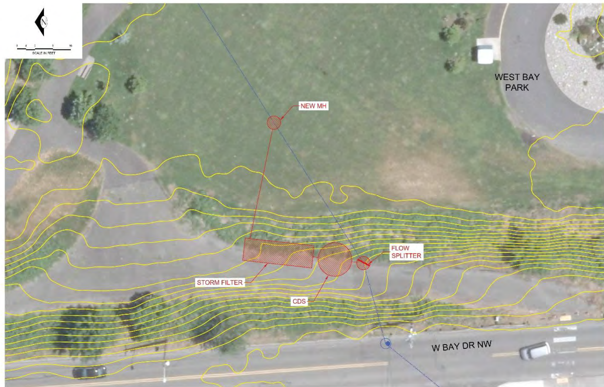
Figure 8 - Example Underground Pretreatment and Filtration Concept at West Bay Park north
